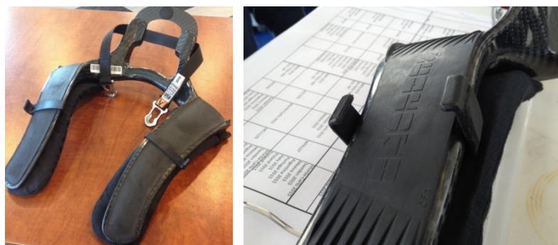
Figure 1 – HANS device with additional small brackets at the bottom of the HANS-yoke
